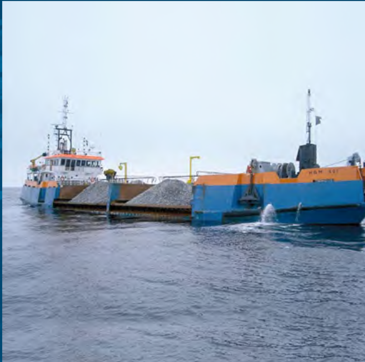
Side stone-dumping vessel HAM 601
